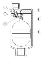
TMO – Max. operating press.: 30 bar; TMO – Max. operating temp.: 300 °C;
